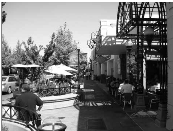
Figure 6.3 The width of the streetside should be planned to accommodate the activities generated by the adjacent land uses. Source: Kimley-Horn and Associates, Inc.
