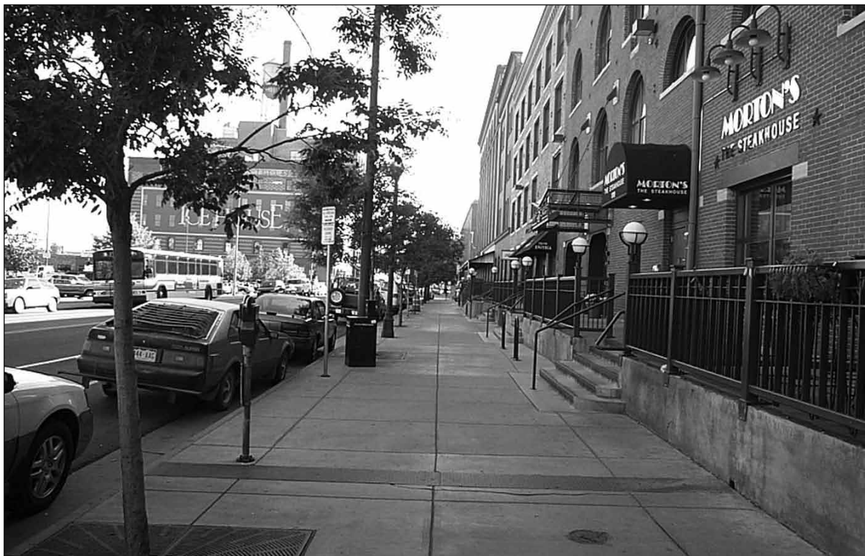
Figure 8.8 A combination of on-street parking, furnishings zone and wide pedestrian thoroughway provides ample buffer from moving traffic. Source: Kimley-Horn and Associates, Inc.
