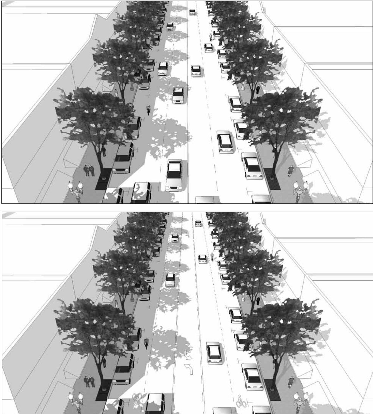
Figure 9.14 Before and after illustration of a road diet. Source: Claire Vlach, Bottomley Design & Planning.
