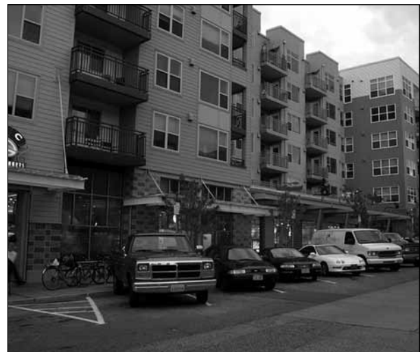
Figure 9.10 Reverse (back-in) angled parking improves driver visibility of bicyclists. Source: Dan Burden, walklive.org.
